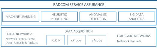
RADCOM Service Assurance: A fully containerized assurance solution that smartly collects and correlates data via multiple sources (network events, Event Detail Records and network packets) for full visibility into the 5G core.
