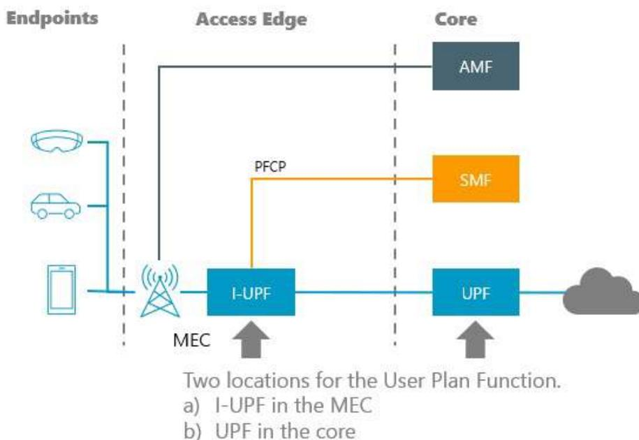
Figure 6 – The UPF function is in the edge (I-UPF) and core network
