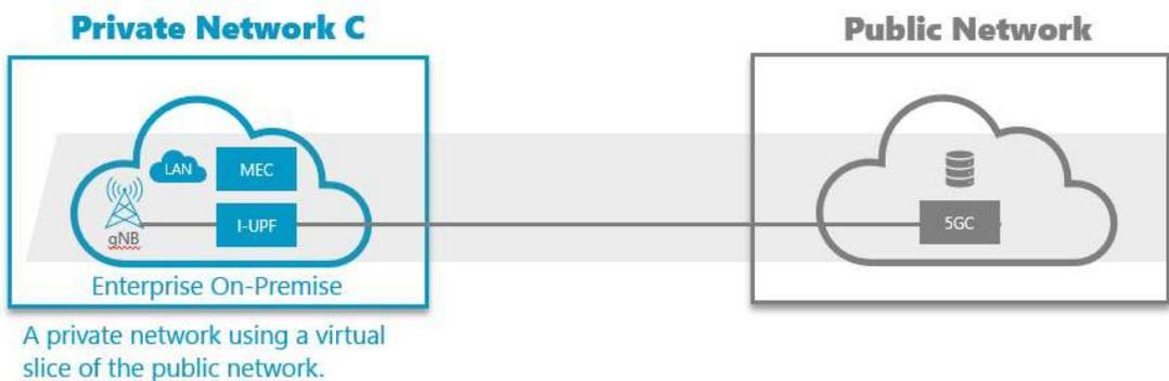
Figure 3 – Network slicing offers a private network as a virtual slice running on the public network
