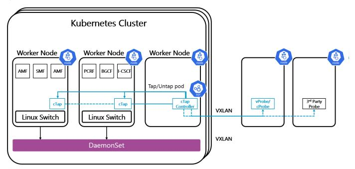
RADCOM cTap can be deployed, controlled, and scaled automatically via Kubernetes' network orchestration integration. It learns the network topology via integration into the Kubernetes API by utilizing RADCOM's controller auto-service discovery via the 5G NRF function. The solution automatically recognizes new network functions and services.
