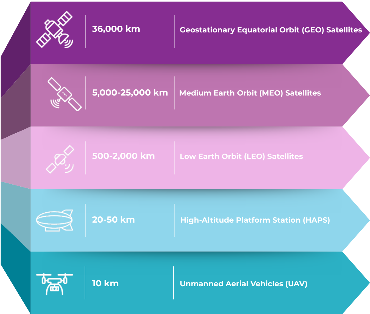
Figure 1: Satellites, UAVs, and HAPS can extend network coverage
